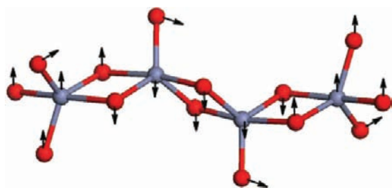
Figure 5. Atom eigenvectors for the vibrational modes of B_g at 11.7i\text{ cm}^{-1} in ZnO_x groups of “ cs\text{-KZnB}_3\text{O}_6 ” (gray and red spheres represent Zn and O atoms, respectively).
